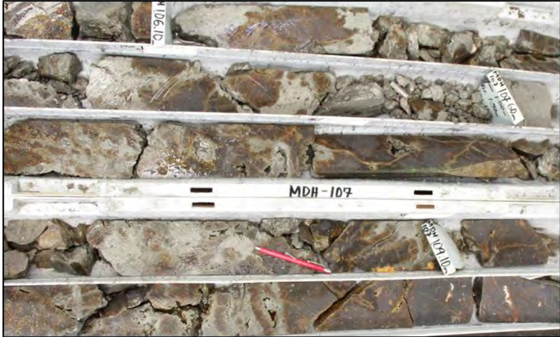
Figure 7.12 Vuggy Silica-pyrite Altered Breccia with Arsenopyrite
